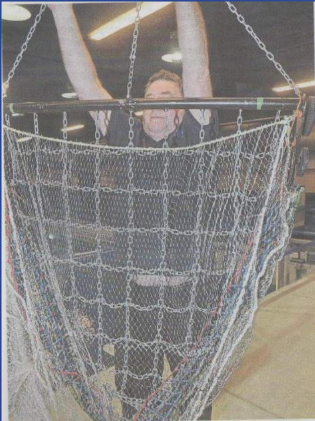
Strong-arm Mike holds up a replica scale model of a conventional beam trawl before it was shot in the tank for comparison alongside the new design of square beam trawl featuring a full-width bosom to help reduce seabed impact and decrease unwanted by-catch of benthic species.
